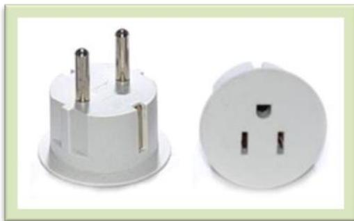
Since the product is already compatible with the local electricity, all the adapter does is allow the prongs to fit the electrical outlets. If you use an adapter with a product that is not dual voltage, you will not only damage your product, but you may also cause electrical damage to the building.
